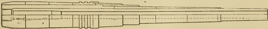
U S Naval 1100pdr 13in Rifle, Breech-loader Weight 60 tons, Muzzle Energy, 33627 Foot-tons
